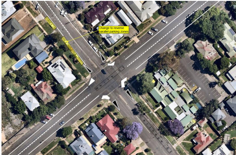
Figure 2: proposed intersection kerb blisters and line marking
